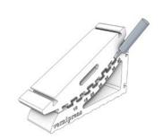
Two models of special anchors guarantee the anchoring of the panels to the concrete support. Extreme anchorage [4 units per row], for the beginning and the end, and a **central model** for the supports that join two panels [2 units per panel].
